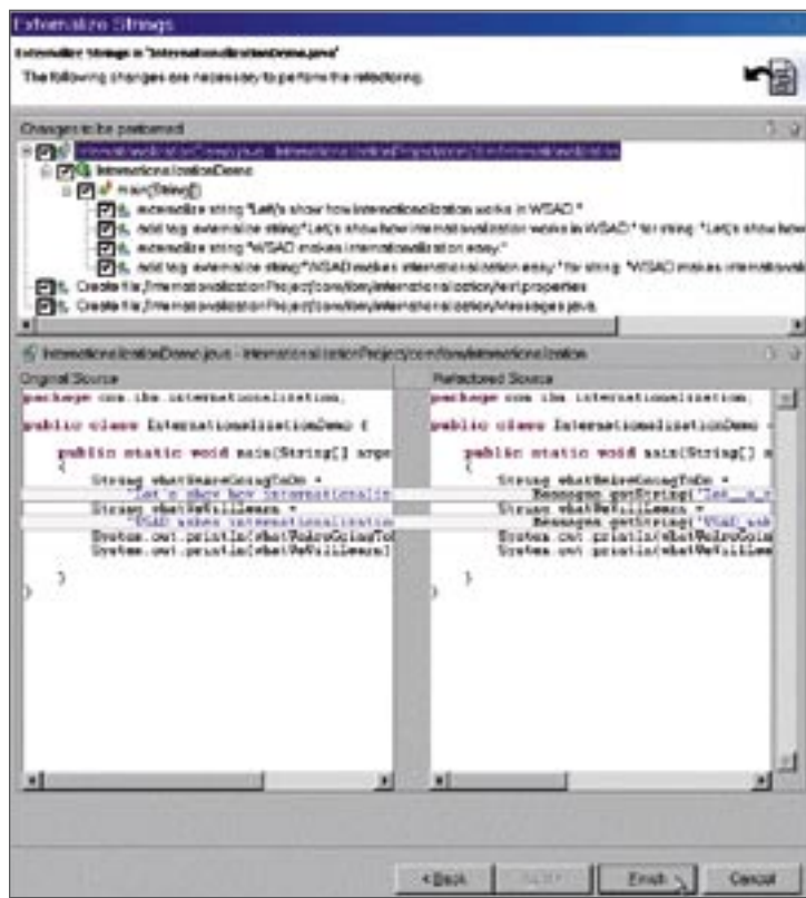
FIG 2: REVIEWING THE PROPOSED CHANGES BEFORE REFACTORING
